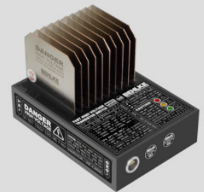
4) HTS 101-03 with nickel plated copper fins (CF)
