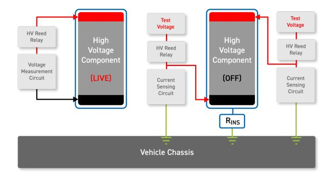
Figure 1 Voltage measurements (on the left) require connecting to a component (such as battery pack terminal) that could be at more than 400VDC. An insulation test (on the right) involves injecting a high voltage into a component and measuring the current that flows through a resistor of a known value (within the current sensing circuit) to the chassis. From that current, the insulation resistance ( $R_{INS}$ ) can be deduced.
