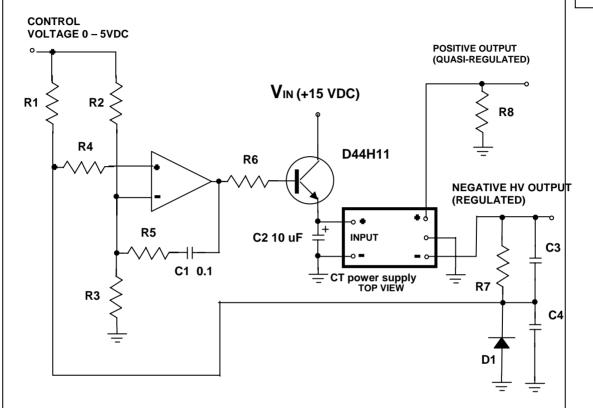
Figure 3: +/- 500 Volt Regulator (Negative output regulation)
