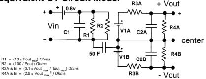
C1 =  $(10 \times 10^{-6})$  Farads C2A & B =  $(0.005 \times lout_{max} / Vout_{max})$  Farads V1 =  $(VR2 \times Vout_{max} / 24)$  Volts
