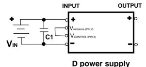
Figure 1: Basic D hookup schematic for maximum output
