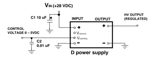
Figure 2: Voltage programming
