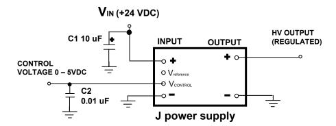
Figure 2: Voltage programming
