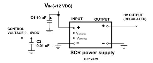
Figure 2: Voltage programming
