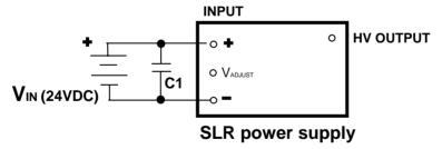
Figure 1: Basic SLR hookup schematic for maximum output
