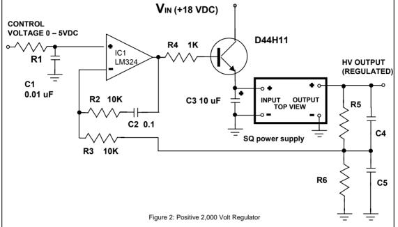
Resistor R2 and capacitor C2 provide frequency compensation for the amplifier IC1 a common bipolar amplifier is used since its outputs and signal inputs can reach almost to ground. R3 provides protection to the signal inverting input of the opamp in case of a short circuit or arcing condition exists on the HV output. R4 protects the output of the opamp in case of a shorted NPN transistor. Typical values for an 2,000 volt Micro channel Plate power supply are as follows:
