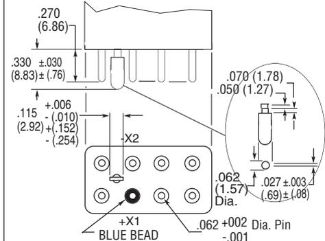
**CODE "G" Circuit Board Pins 28 VAC Coils**
