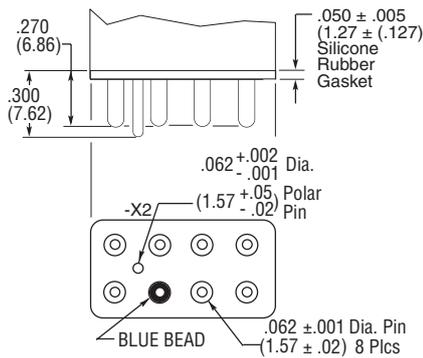
**CODE "B" Circuit Board Pins - All DC Coils**
