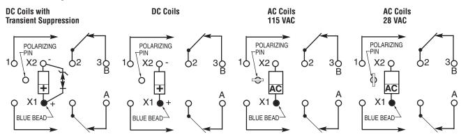
NOTE: Polarity must be observed with DC coil supply. Relay is polarized with a permanent magnet and will not operate or be damaged by reverse polarity.
