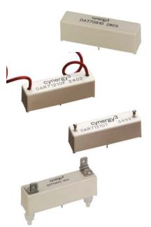
Very high isolation voltages, up to 15kV, are achieved through the use of high vacuum reed switches with either rhodium or tungsten contacts and make these relays suitable for high reliability applications, such as cardiac defibrillators, test equipment and high voltage power supplies.
