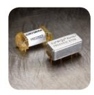
A latching RF reed relay designed for manpack, portable HF radio systems, from 1-30MHz, where power resources are limited and board space is at a premium. These relays have separate set and reset coils to simplify board design, are capable of carrying up to 1.5A current at 30MHz and can withstand either 1.5, 3 or 3.5kV between contacts. The FRS22012 is a fast latching relay with RF and magnetic screening, that enables switching with coil pulse lengths down to 0.5ms.
