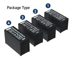
The Pickering Series 100 is a complete range of Single-in- Line (SIL) reed relays primarily intended for direct drive from 4000B CMOS or NMOS logic or similar low current sources. The mercury wetted relays in the range may be driven directly from TTL logic.
