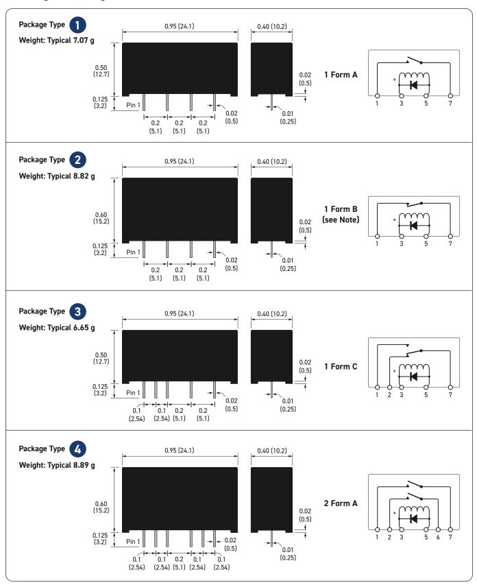
Pin Configuration, Weights and Dimensional Data (dimensions in inches, millimeters in brackets)
