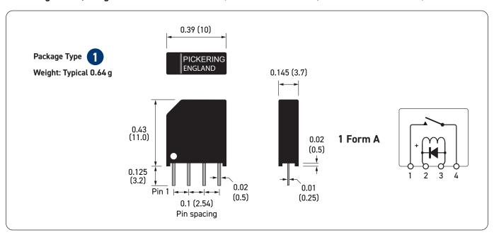
**Important:** Where the optional internal diode is fitted the correct coil polarity must be observed, as shown by the + symbol on the schematics.
