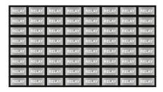
In this small area of only  $2.16 \times 1.2$  inches  $(5.48 \times 3.05 \text{ cm})$ , it is possible to construct an  $8 \times 8$  matrix - 64, 1 Form A relays.
