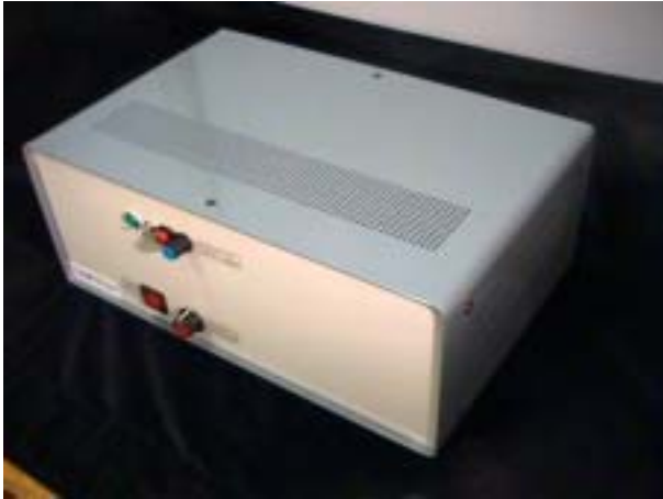
A three output, variable risetime insulation tester.
