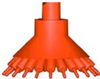
3-D Model of the high voltage electrode in a corona stabilised switch, created to evaluate the field of the critical volume region.
