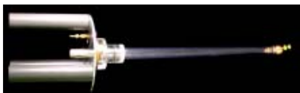
A 200kV liquid resistive probe DE(LRP)-01. The input impedance is 2k \Omega , and the response time is down to 5ns.
