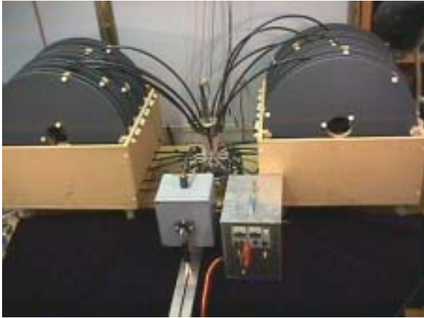
A self-matched pulse generator in use driving a flash lamp load for electronic pasteurisation experiments.
