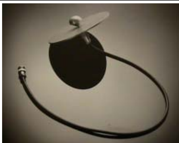
A conical D-dot probe complete with signal cable, and designed to match into standard 50Ω cable.
