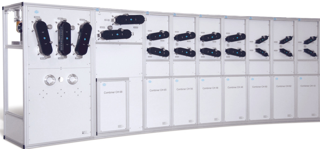
BN 575306 Turkmenistan UHF combiner for 8 x 4 kW DVB with integrated mask filters, combiner bypass and antenna patch panel with bent front for installation in circular transmitter hall
