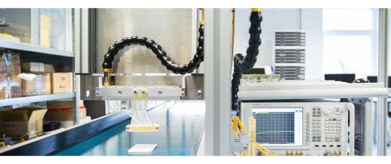
**SPINNER EasySnake** for E- and W-band performs the function of a **hollow metallic** waveguide but offers two degrees of freedom: flexible bending and twisting **in any direction** while delivering excellent measurement results at the same time. Even conventional flexible waveguides made of electrically conductive bellows are typically non-twistable i.e. resist torsion, which significantly limits the feasible test configurations.
