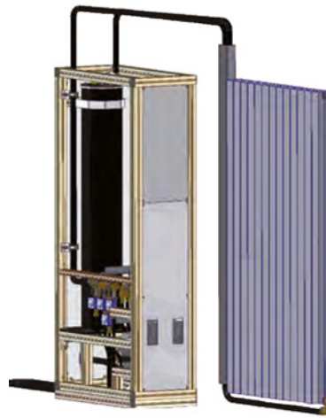
Pump unit and indoor cooler
