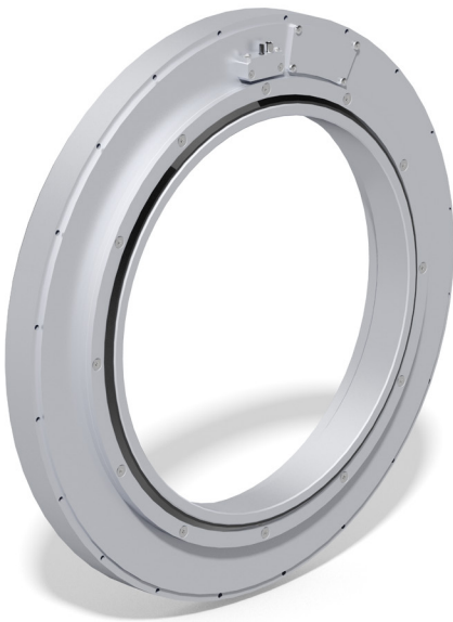
SPINNER contactless capacitive rotary joint for GigE (1000Base-T) or 100 Mbit/s real time transmission with 300 mm inner clear diameter (BN 637418C000X)
