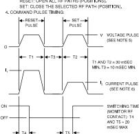
5. COMMAND SWITCHING VOLTAGE: V = 26-32 VDC PULSE
