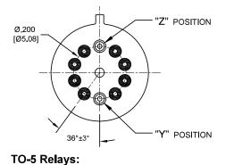
ER412, ER412T, ER422, ER432, ER432T, 712, 712TN, 400H, 400K, 400V, RF300, RF303, RF341, RF312, RF332, RF310, RF313, RF320, RF323, Indicates ground pin position
