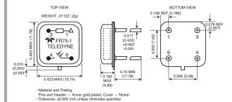
Figure 1 – FR75-1 mechanical specification; dimensions in inches (mm)
