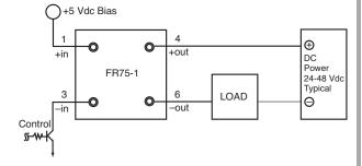
Figure 5 — FR75-1 typical wiring diagram
