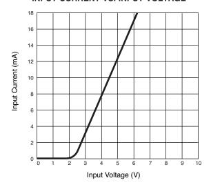
Figure 2 — FR75-1 input current vs. input voltage
