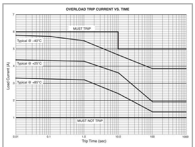
Figure 6 — FR75-1 overload trip current vs. time
