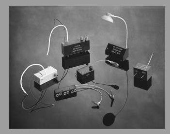
Micapacitors in Voltage Multipliers Raw Micapacitors are used in Reynolds Micaplier voltage multipliers. These units have output voltages ranging to 160 kVDC. Micapliers are used in a wide range of military and commercial applications. Typical applications are: CRT anode and focus supplies for airborne EFIS (Electronic Flight Instrumentation Systems), X-Ray equipment and low power (mini) TWT's.
