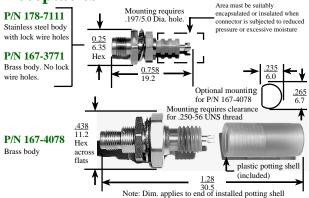
P/N 178-7111 Front mount, non-sealed connector. Stainless steel body. Lock wire holes
