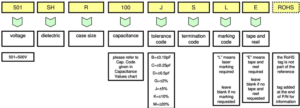
NB: for capacitance values lower than 10pF, tolerances B, C and D apply. For capacitance values equal to or higher than 10pF, tolerances G, J, K and M apply.
