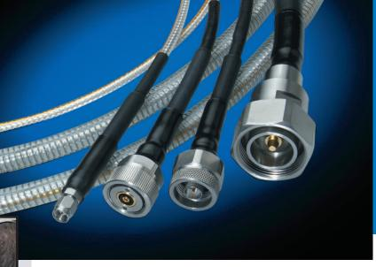
SilverLine  $^{\circledR}$ -SF (Super Flex) SilverLine  $^{\circledR}$ -SF is approximately 40% more flexible than traditional SilverLine  $^{\circledR}$ . This is accomplished by replacing the steel center conductor with copper and the FEP outer jacket with polyurethane. SilverLine®-SF retains its bent shape. That is, the cable has memory.
