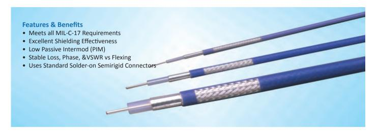
TFlex® employs a thin helical wrap of silver plated copper tape and overall braid sized such that standard solder-on connectors can be used.
